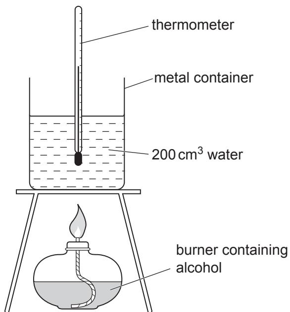
The student determines the temperature rise of 200 cm<sup>3</sup> of water when an alcohol burns.
