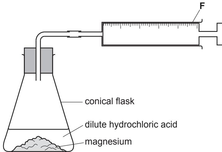
In each experiment the student adds dilute hydrochloric acid to magnesium. The volume of hydrogen in apparatus **F** is recorded every 30 seconds.
